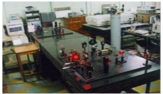
A view of the set up for thermal lens studies using the OPO as the pump source.
